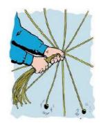
The bunch connector is only intended for use freely hanging on the tunnel face.
