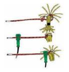
The bunch is passed through the loop of 5 g/m detonating cord. A SnapLine 0 is fitted to the loop and slid towards the bunch.
